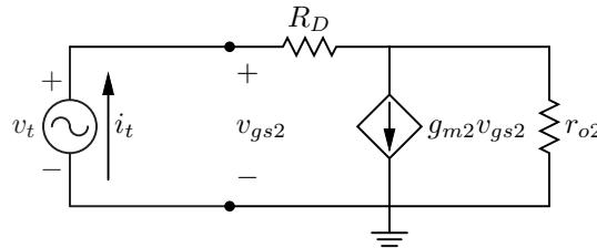
$$i_t = g_{m2}v_{gs2} + \frac{v_t - i_t R_D}{r_{o2}}$$
