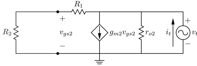
$$i_t = \frac{v_t}{R_1 + R_2} + g_{m2}v_{gs2} + \frac{v_t}{r_{o2}}$$
