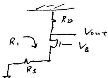
$$R_{out} = R_D // R_L \\ = R_D // [(1 + g_m r_o) R_s + r_o] \\ \text{(from Eq. (7.110))} \\ \approx R_D // (g_m r_o R_s + r_o) \quad (\because g_m r_o \gg 1) \\ = \frac{g_m r_o R_s R_D + r_o R_D}{R_D + g_m r_o R_s + r_o}$$
