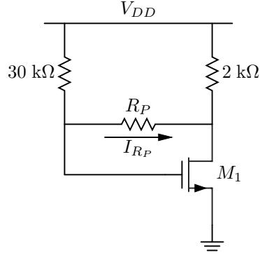
$$V_{GS} = V_{DD} - I_{R_P}(30 \text{ k}\Omega)$$
