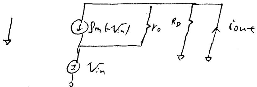
$$g_m = \frac{i_{out}}{V_{in}} = g_m + \frac{1}{r_o} \\ \approx g_m \quad (\because g_m r_o \gg 1)$$
