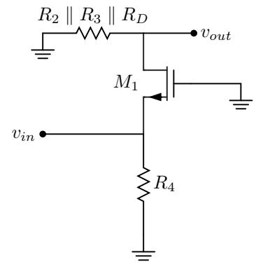
$$A_v = \boxed{g_m (R_2 \parallel R_3 \parallel R_D)}$$
